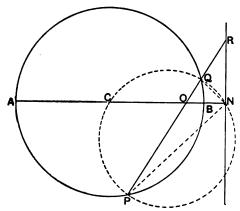
Let PQ be any chord of a given circle which passes through the given point O, and let R be the harmonic conjugate of O with respect to the points P, Q.
